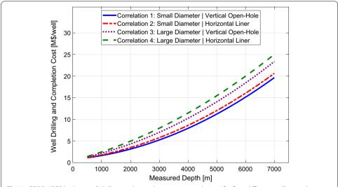
**Fig. 3** GEOPHIRES built-in well drilling and completion cost correlations for four different well types (Lowry et al. 2017). Small and large diameter refers to 8½-in. and 12¼-in. bottom-hole diameter. Plotted cost data includes 15% contingency, but excludes indirect costs
