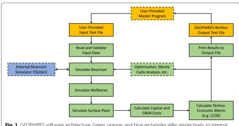
**Fig. 1** GEOPHIRES software architecture. Green, orange, and blue rectangles refer, respectively, to internal GEOPHIRES components, external user interface components, and the external reservoir simulator TOUGH2
