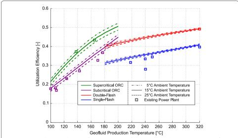
**Fig. 2** GEOPHIRES built-in utilization efficiency correlations for ORC (subcritical and supercritical) and flash (single and double) power plants. Correlations provide power plant utilization efficiency as a function of production and ambient temperature
