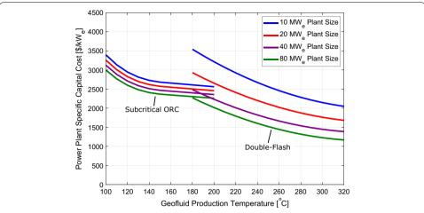
**Fig. 4** GEOPHIRES built-in capital cost correlations for subcritical ORC and double-flash power plants. Plotted cost data includes 15% contingency, but excludes indirect costs
